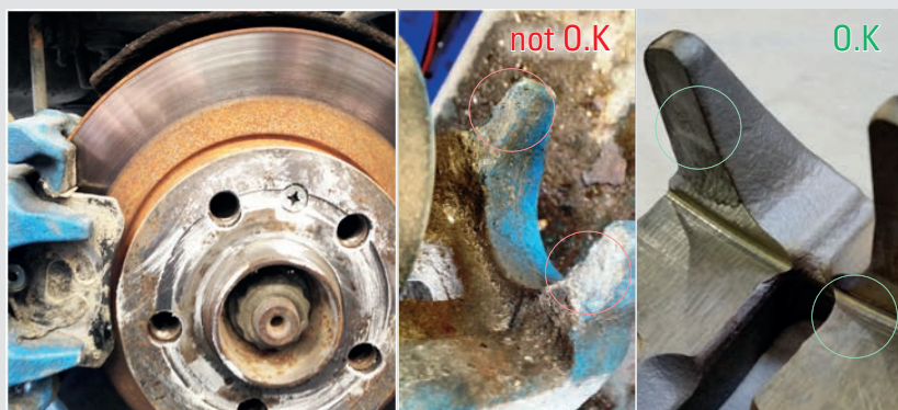
► Uneven wear pattern on the brake disc
